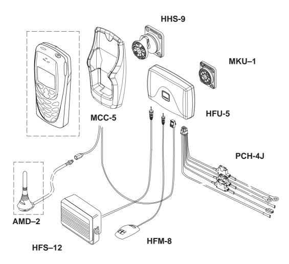
Please, note that the items enclosed in broken-line (phone & antenna) are not supplied with CARK132. The external antenna AMD–2 is recommended.
